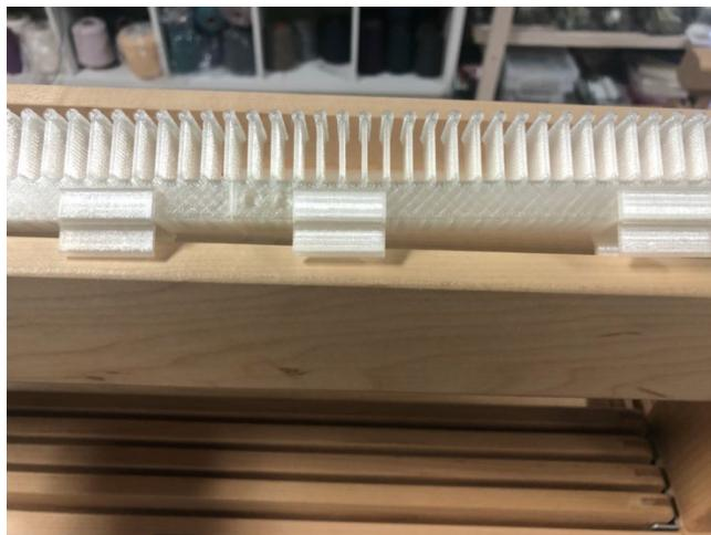
To attach your raddle, first assemble the raddle sections by pushing firmly at the joins. Next place about 2 clips on each 6-inch section.
